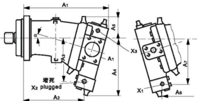
A<sub>1</sub> 和 X<sub>3</sub> 仅用于带压力切断 A<sub>1</sub> and X<sub>3</sub> with pressure cut-off only
