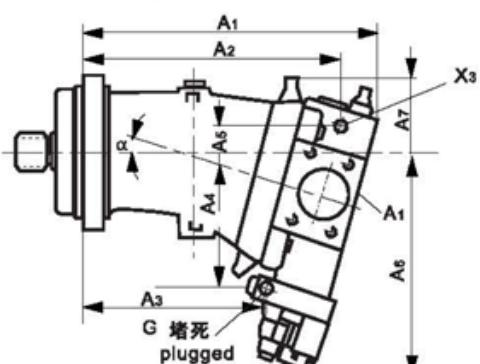
A<sub>1</sub> 和 X<sub>3</sub> 仅用于带压力切断 A<sub>1</sub> and X<sub>3</sub> with pressure cut-off only
