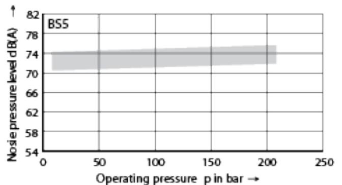
The noise pressure levels for double pumps lie on average 1 to 3 dB(A) above the values for single pumps.
