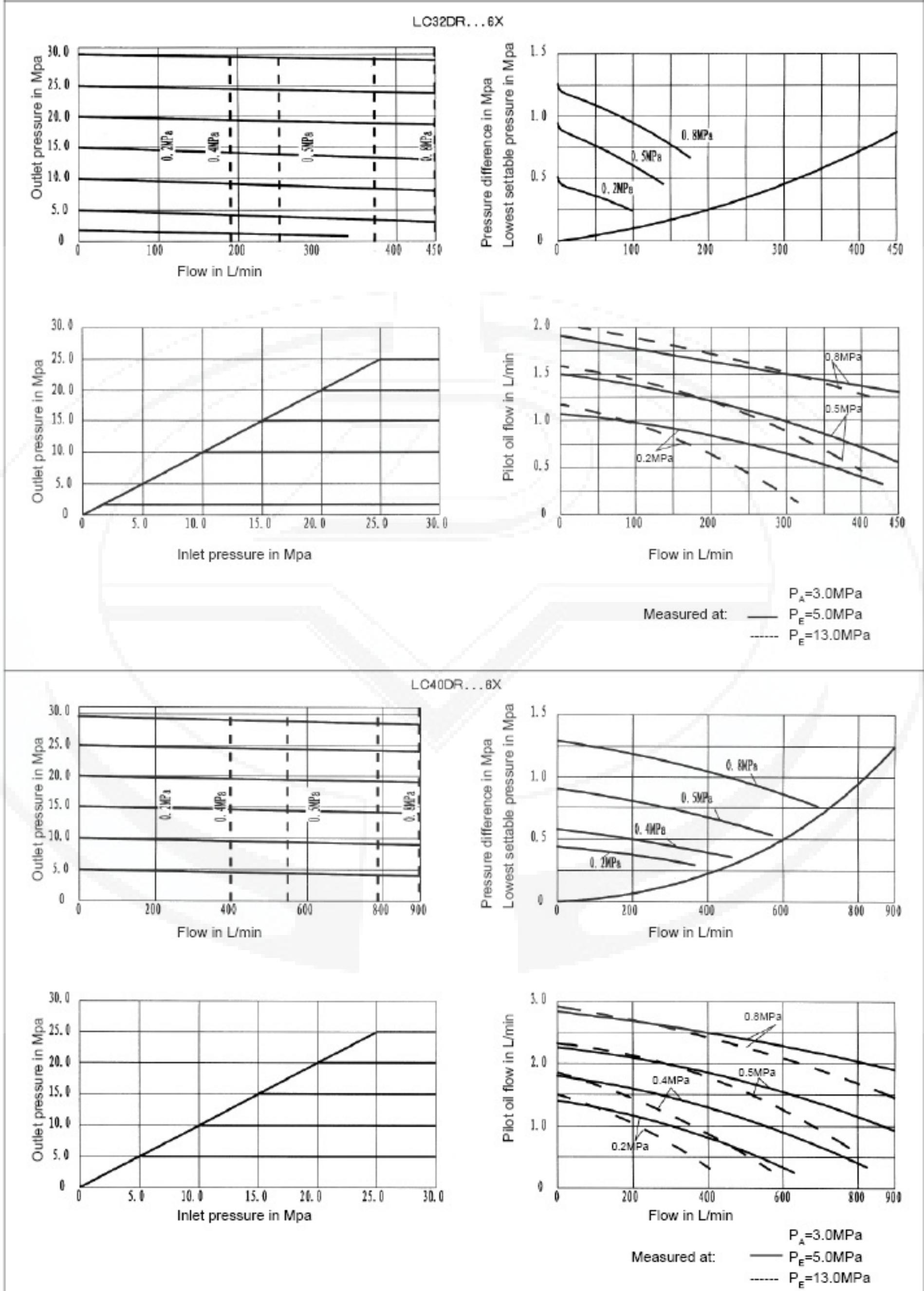
**Characteristic curves** (measured at  $v = 41 \text{ mm}^2/\text{s}$  and  $t = 50^\circ\text{C}$ )
