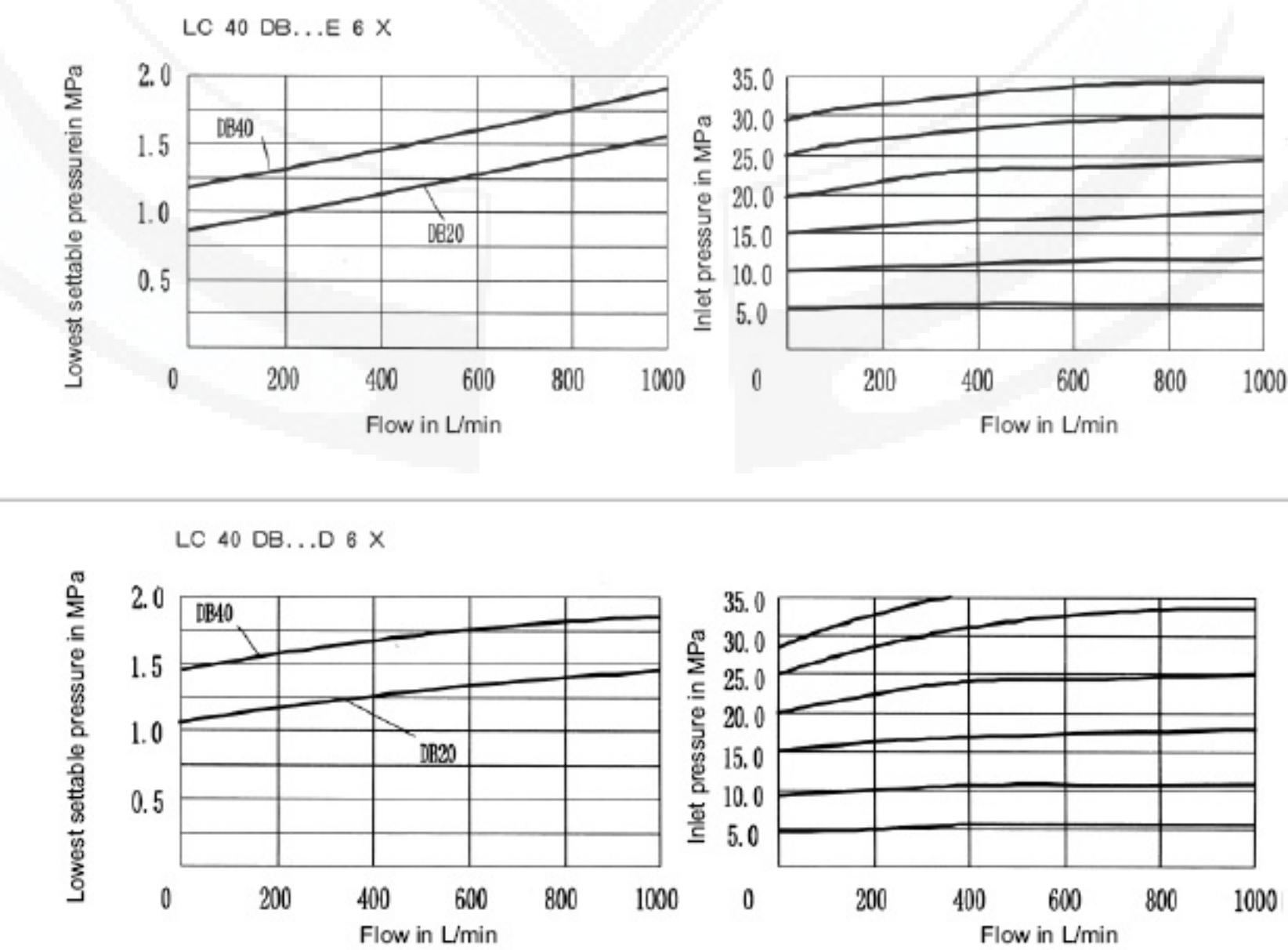
**Characteristic curves:** (measured at  $v = 41 \text{ mm}^2/\text{s}$  and  $t = 50^\circ \text{ C}$ )
