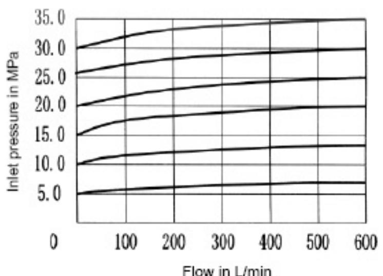
**Characteristic curves:** (measured at  $v = 41 \text{ mm}^2/\text{s}$  and  $t = 50^\circ \text{ C}$ )
