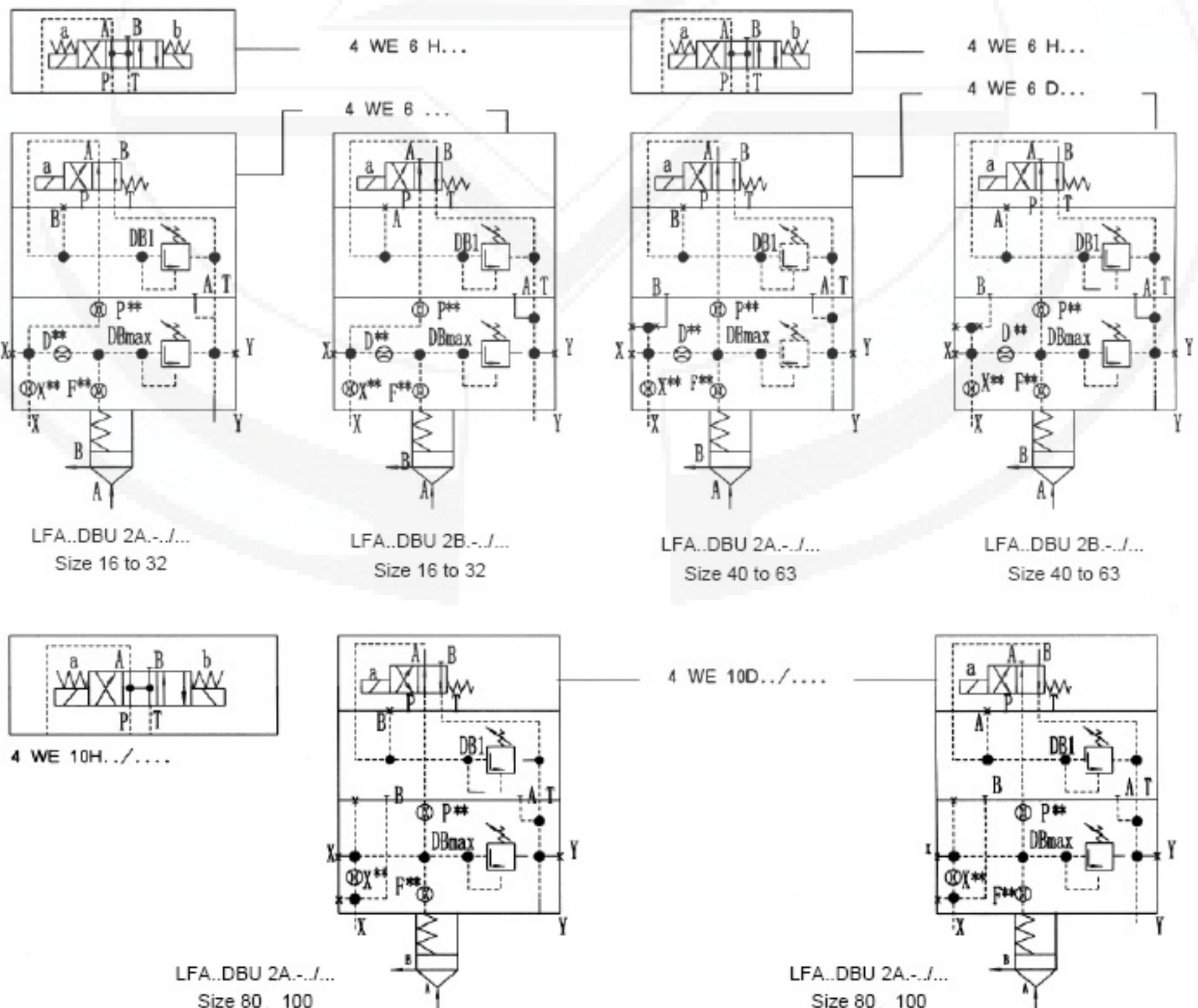
**Control cover with 2 manual pressure adjustment, electrical selectable**
