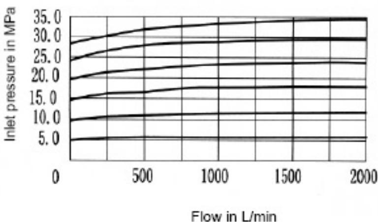
**Characteristic curves:** (measured at  $v = 41\text{mm}^2/\text{s}$  and  $t = 50^\circ \text{C}$ )
