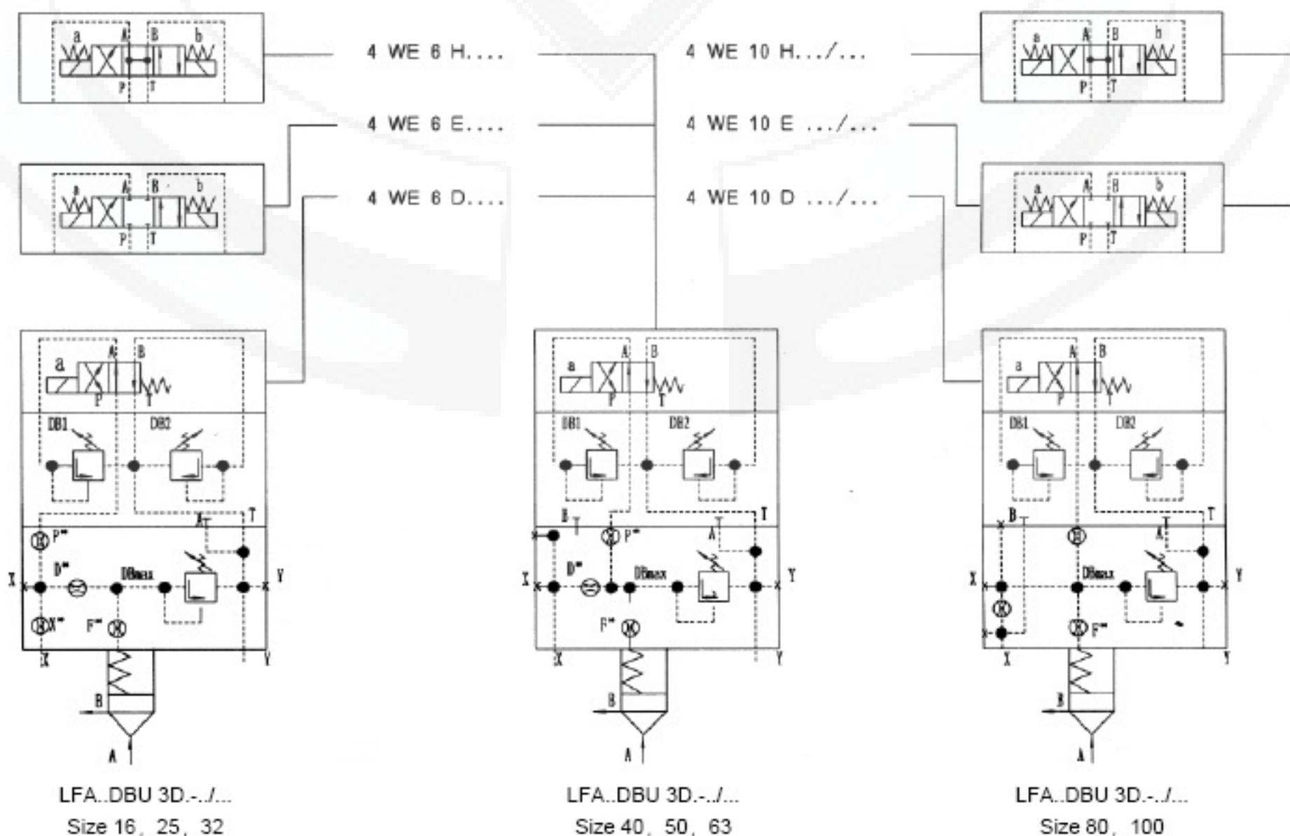
**Control cover with 3 manual pressure adjustments, electrically selectable**
