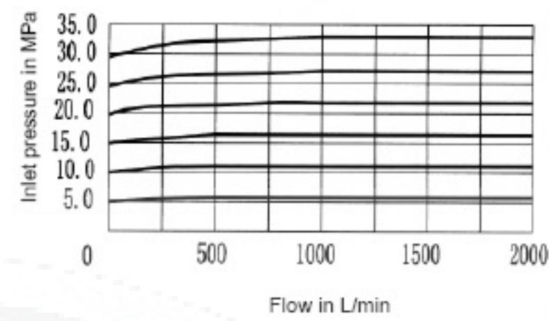
Electrical proportional pressure adjustment, type LFA 50 DBE... 6XB/...
