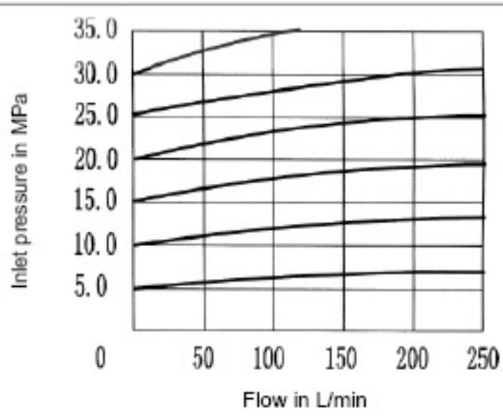
**Characteristic curves:** (measured at  $v = 41 \text{ mm}^2/\text{s}$  and  $t = 50^\circ \text{ C}$ )
