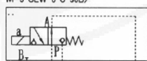
**Control cover with manual pressure adjustment, for electrical unloading**
